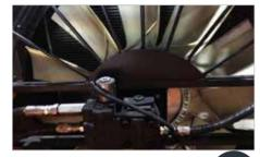
The fan speed varies in accordance with the coolant and brake oil
